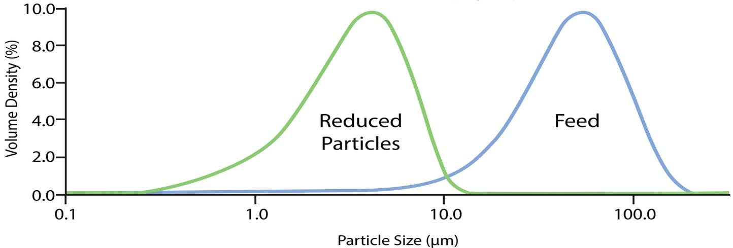
Nutraceutical test: blue curve is the feed, green curve is the micronized product
